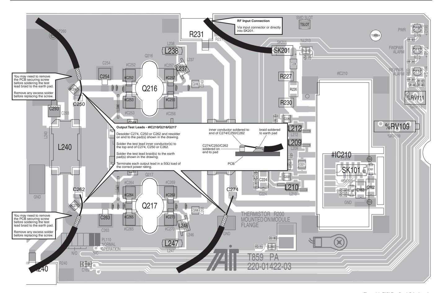
Figure 4.4 T859 Test Break Point Location
