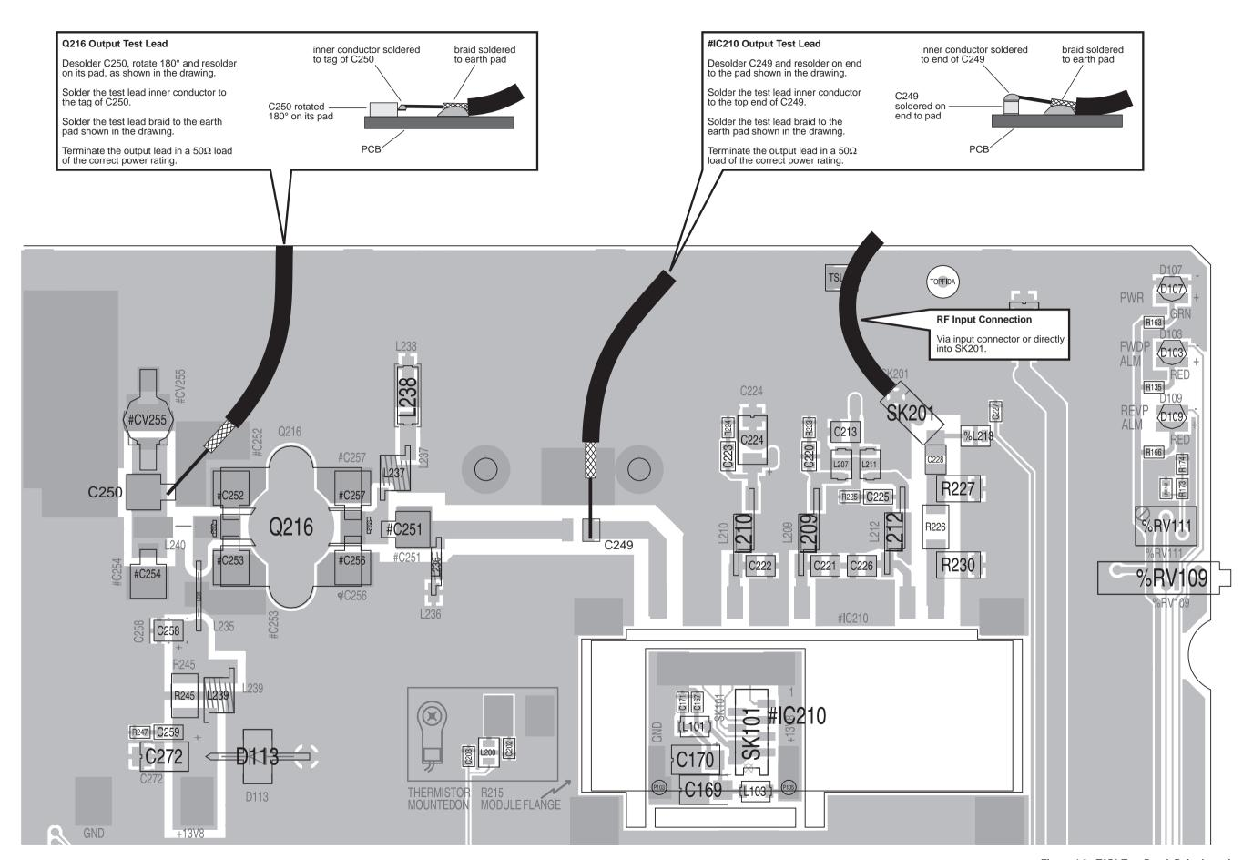
Figure 4.3 T858 Test Break Point Location
